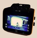
This scanner allows you to view and digitize photo negatives that are in a slide format.
